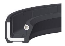
Rotary shaft seals are suited for use on rotating machine elements, such as shafts, hubs and axles. They are used to seal against a wide variety of media statically and dynamically. Typical fields of application include powertrain technology, agricultural and construction machinery, wind turbines, ship-building and other areas of application in the manufacture of machines and devices.
